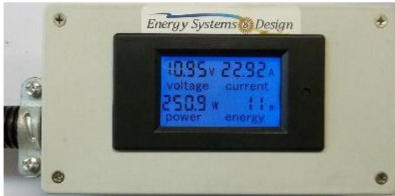
We were making a 30 amp meter for use with hydro machines, or anything else. We now make a 50 amp model for \$99 and a 100 amp for \$119.
