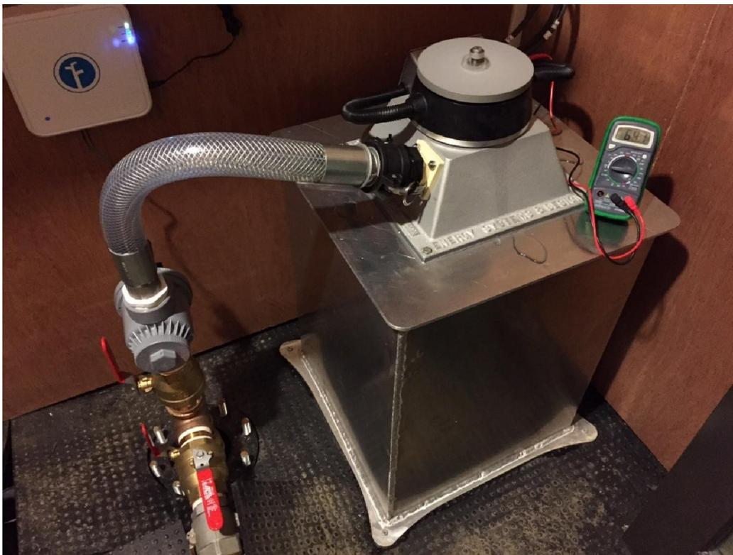
*1 nozzle Stream Engine, High Current (HC) stator with stainless Low Flow (LF) wheel.
