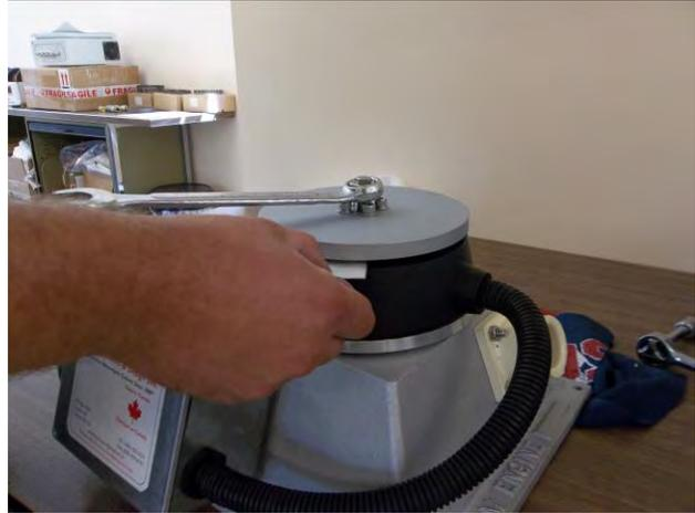
Minimum rotor height air gap at least 0.020" (0.5mm)
