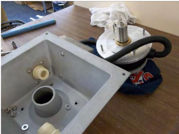
Remove low flow wheel shaft adaptor
