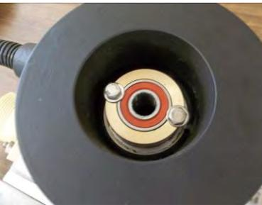
Remove bearing retaining bolts
