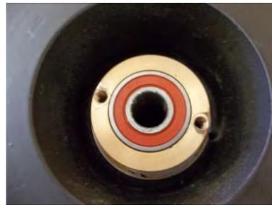
Invert stator to remove bearings
