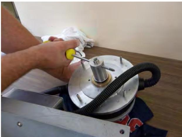
Readjust height of rotor
