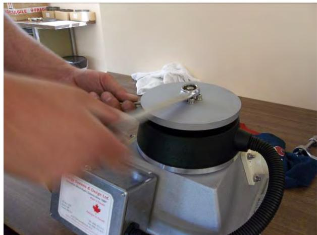
Lowering rotor height and locking in place. Final adjustment for power output should be done after the turbine is reinstalled and the power output is read with the digital multi meter.
