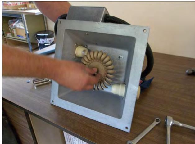
**\*\* Always turn the rotor by hand before starting the machine to check for rubbing\*\*.**
