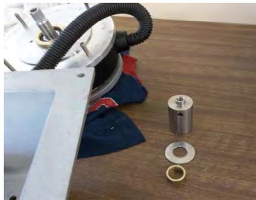
Once either style of wheel is removed the rotor should be raised until the magnetic attraction is low enough to separate the rotor from the stator. This is more easily done if the generator is placed back on the housing.
