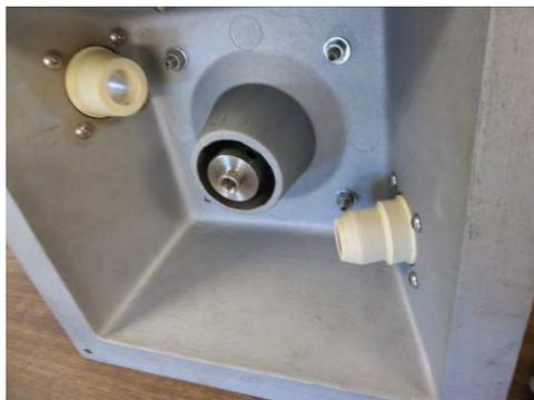
Remove generator mounting nuts and washers
