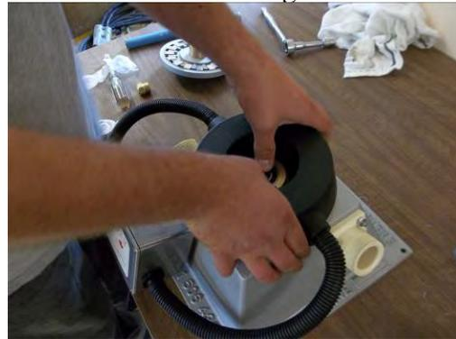
Bearings inserted, reassemble
