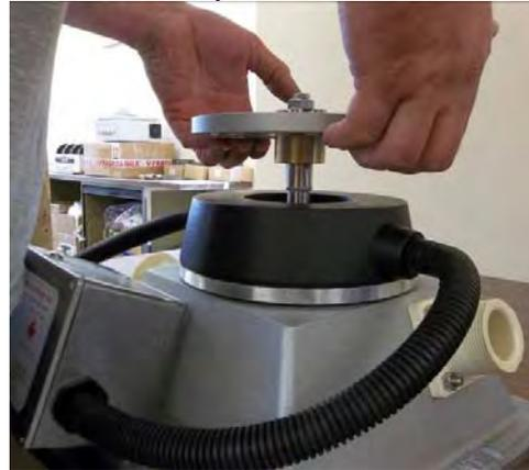
Magnetic rotor shaft hub assembly removed
