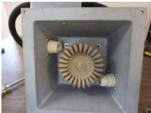
Unscrew center bolt with 9/16"(14mm) socket or wrench
