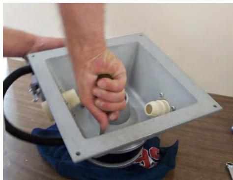
Generator removed for low flow version
