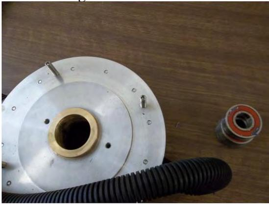
Top side of stator with bearings removed
