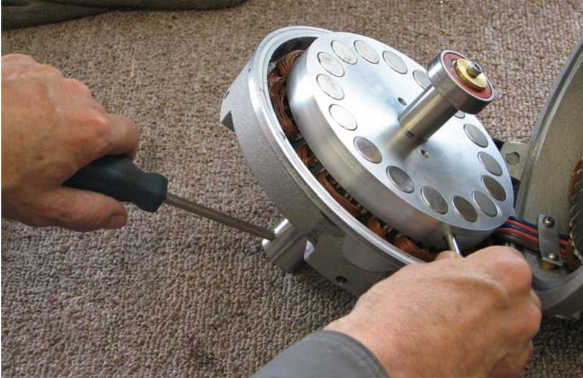
The photo shows how to remove the hub for a machine with a low flow runner.
